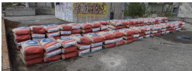
Foto 6. Probni teret ( q_{max} = 300 \text{ daN/m}^2 )
